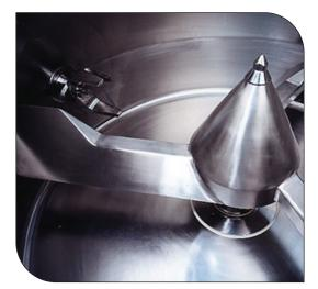
Unique Tangential elevated tip impeller for unique mixing pattern
