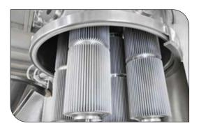
Special CIP SS cartridge filter bag provided for containment application with Air blow cleaning system & auto lowering with pneumatic telescopic cylinder
