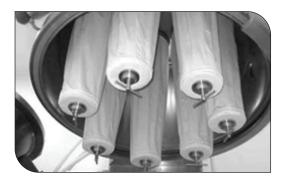
Antistatic Finger provided option for Single Bag Shaking & Twin Chamber Bag Shaking System.
