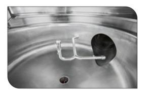
Tangential inlet air in plenum for spiral air flow gives uniform core drying. This also avoids rat hole formation eliminating need for racking and stopping fluid bed process before completion.
